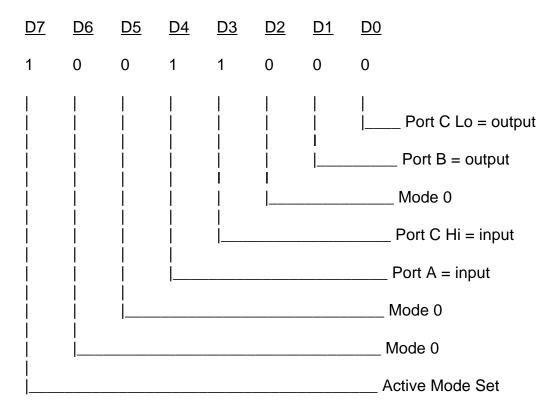
This corresponds to 98 hex. If the card base address is 2D0 hex, use the C command to write to the control register as follows:
